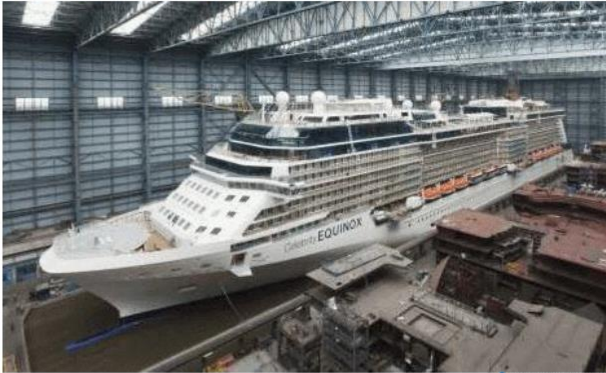
CLEAR SPAN 111.85 m, HEIGHT 74.84 m LENGTH 503 m. SOURCE: MEYER WERFT BROCHURE – PAPPENBURGH SHIPYARDS, GERMANY
